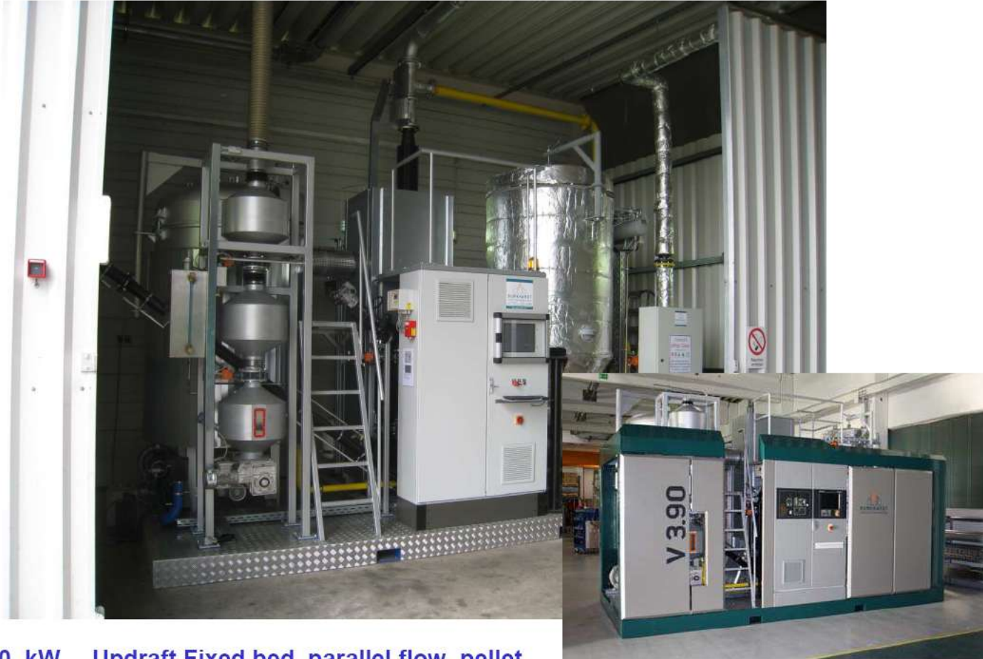
200 kW el . Updraft Fixed bed, parallel flow, pellet,
